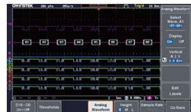
Display analog waveform converted from digital signal
