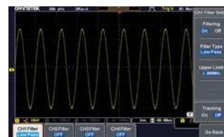
Filtered Waveform, Noise Removed
