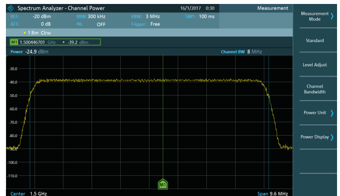
R&S®FPC-K55: channel power measurement
