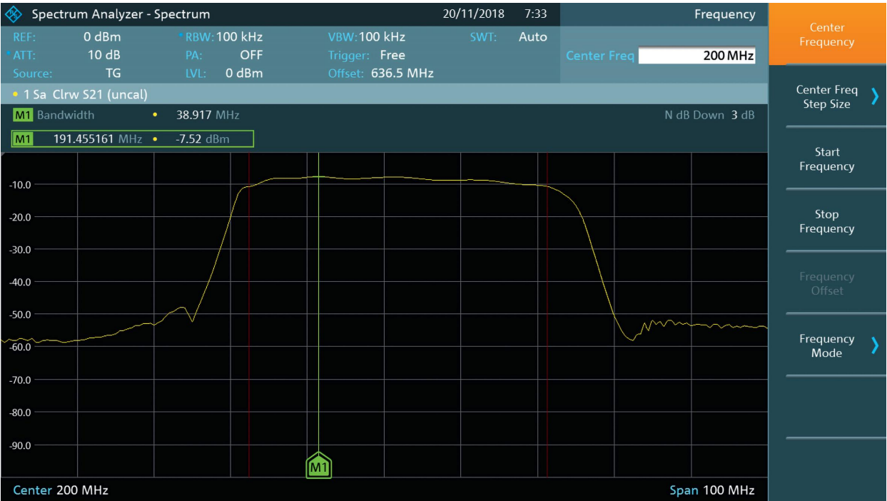
R&S®FPC1500: tracking generator measuring signal chain containing mixers, filters and amplifiers
