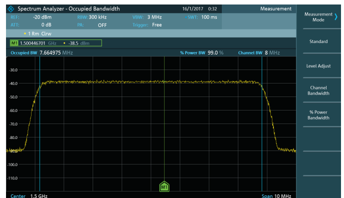
R&S®FPC-K55: occupied bandwidth measurement
