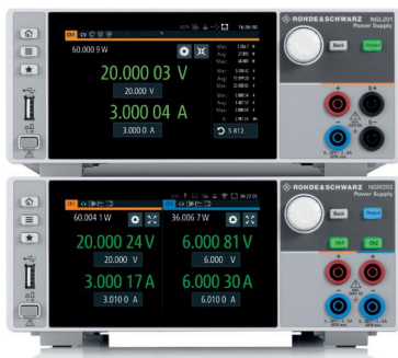
R&S®NGL201 single-channel and R&S®NGM202 two-channel power supply
