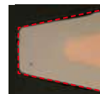
Weller WSW after 10,000 solder cycles
