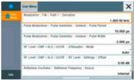
Example of a user menu; individually composed parameters can be directly set in this menu
