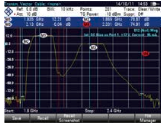
Two-port capability for transmission measurements
