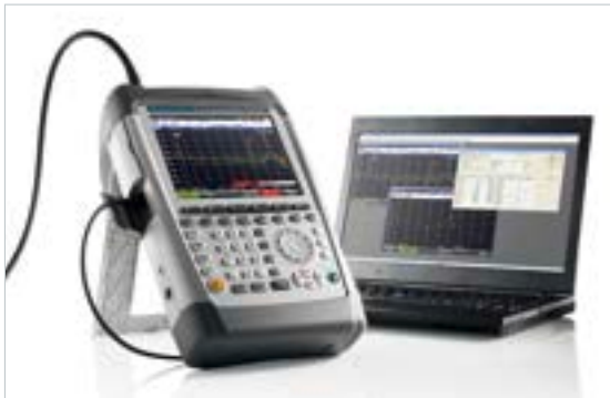
Vector network analysis: Simultaneous display of four S-parameters ( S_{11} , S_{21} , S_{12} , S_{22} )
